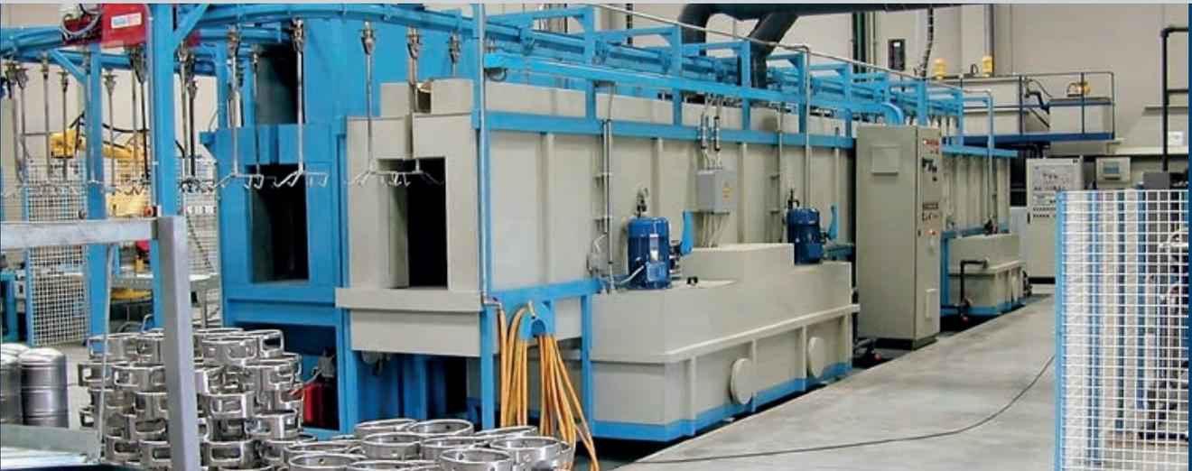
When using photocells at the tunnel entrance, the PLC switches off in sequence the different zones, with greater energy saving.
